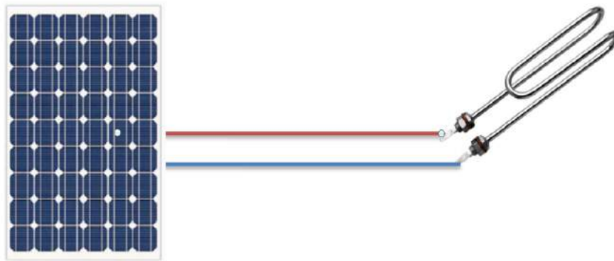
Fig. 1. Example of the system directly supplying loads Source: own development
